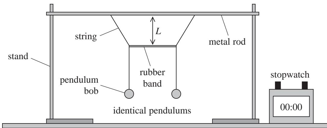
One pendulum is set in motion. The amplitude of oscillation of this pendulum decreases to zero as the rubber band transfers energy to the other pendulum, which oscillates with increasing amplitude.
